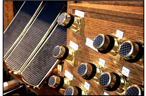
Toe pistons with felt bushings and expression pedals with the correct amount of drag simulating operation of swell shades.
