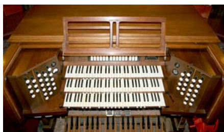
The finished console. All new walnut stop jambs, coupler tab rail and thumb piston rails, as well as all new hardware.
